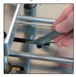
Unhook the nylon cord and gently let the spring push the strip of wedges into the magazine. Use visual observation to confirm that the wedges slide under the cap with a gap of no more than 0.5mm.
