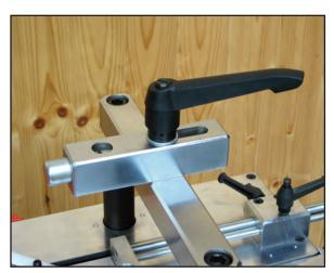
Push the adjusting button inwards and insert, from above, the Vertical Bar (C).
