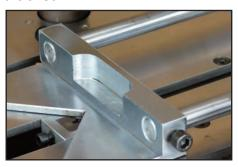
Fit the Handle and Locking Collar (Q) over the right hand fence bar.
