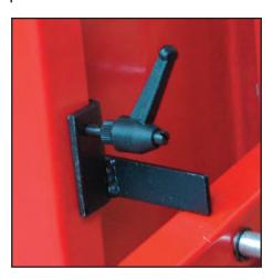
The Locking clamp can also be used to lock the footpedal half way down, This reduces the amount of travel required to insert a wedge and is sppeds up th epinning operation when working with small mouldings.
