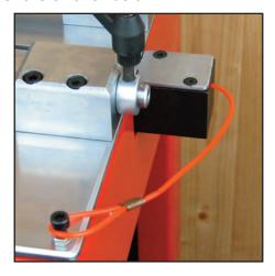
Insert a strip of wedges, sharpened side upwards. When using genuine Framers Corner Wedges, insert with glued side up.
