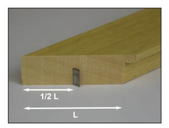
When inserting 2 or more wedges into a corner the first position should be 1/4 distance from the front edge. The last position should be 1/3rd distance from the back edge.
