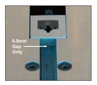
To remove wedges from the magazine, reverse the proceedure.
