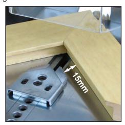
Release the foot pedal and the clamp will move forward, gripping the moulding. The tip of the clamp is desgined to allow for slight variations in the moulding width.
