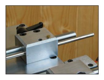
Place the Brass Nipple (S) into the threaded hole in the fence block.
