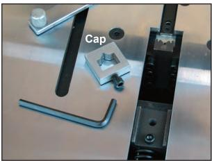
To clear a blockage; remove the cap, using the hex key provided. Once removed, the driver should drop back down and the jammed wedge can easily be removed.
