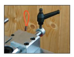
Insert the Front Stop Bar (A) into the hole in the fence block.
